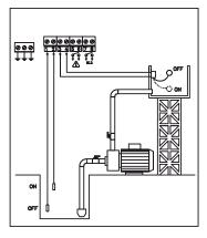
further applications: sewage disposal, rain water harvesting, dry run protection for impeller pumps
